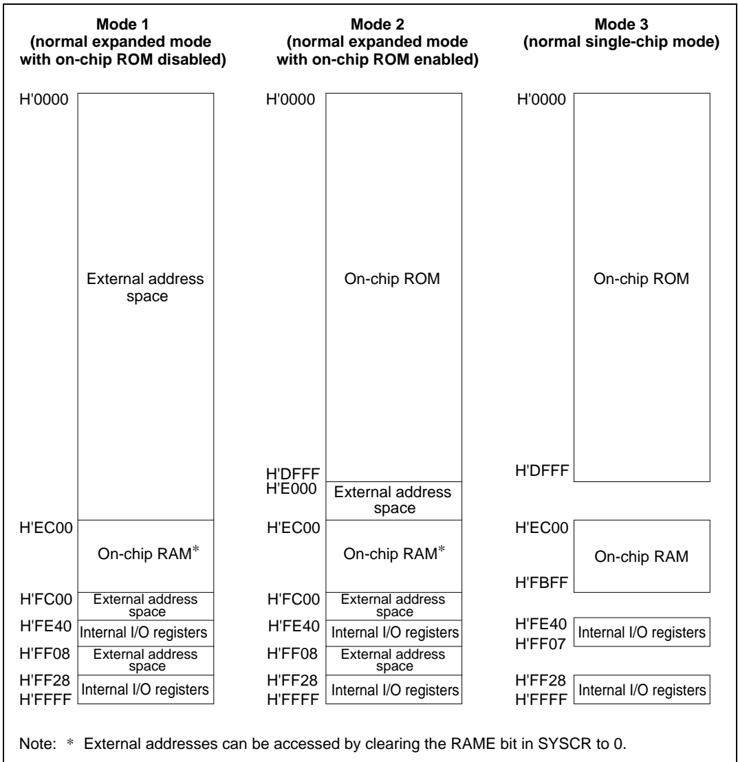
Figure 3.2 Memory Map in Each Operating Mode in the H8S/2344
